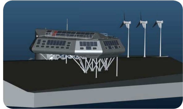
Figure 2: The wind conductor can be seen clearly under the rear side of the station.
